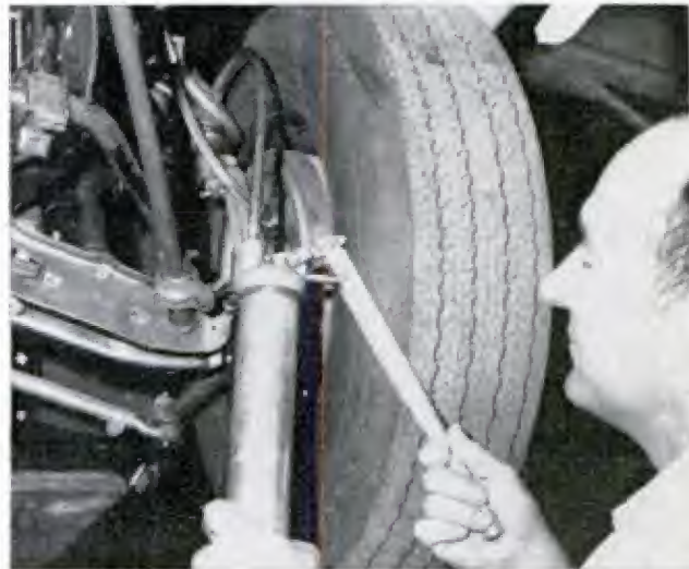
CHASSIS LUBRICATION can be done with inexpensive grease gun; the cartridge-fill type is the easiest
